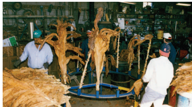
Figure 8. Stripping-wheel tobacco stripping aid.
