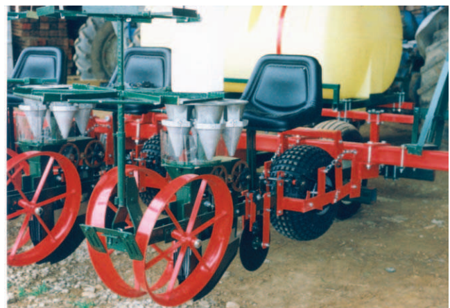
Figure 6. Carousel transplanter used for transplanting tobacco seedlings produced in float trays.
