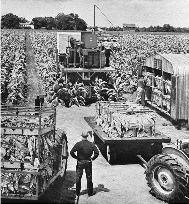
Figure 9. Picture from a Powell Manufacturing Company ad from about 1968 showing their prototype mechanical harvester and commercial bulk curing barn.
