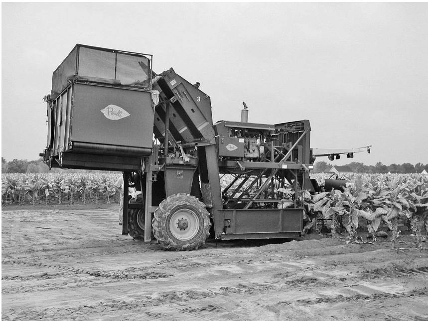
Figure 19. Modern 2-row mechanical harvester with live bottom collection bin entering a field.
