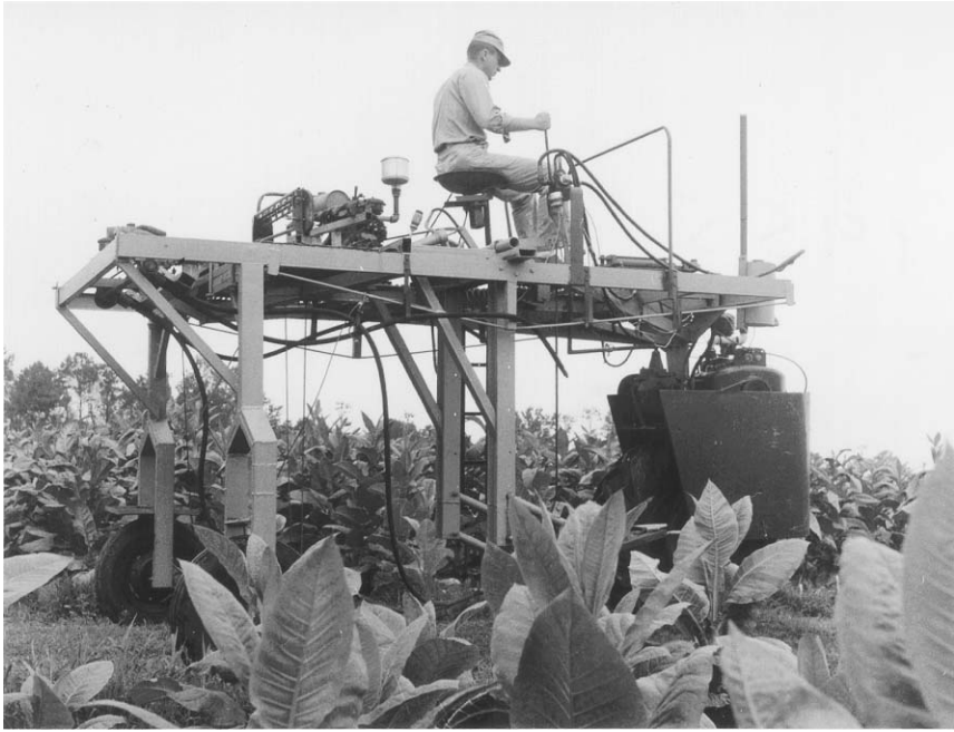
Figure 7. Graduate student Charlie Suggs operating an early prototype of the mechanical harvester developed by North Carolina State University.
