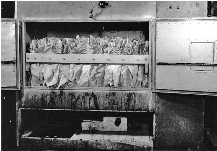
Figure 11. Experimental bulk-curing chamber using new rack design to hold leaves for curing at Oxford Tobacco Research Station in 1957.
