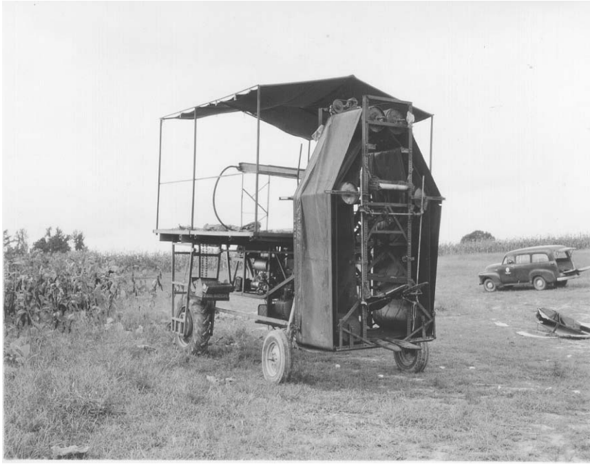
Figure 8. North Carolina State University prototype mechanical harvester with early belt conveyor design.
